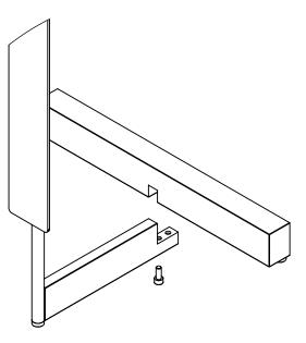
Fasten the base with the screw provided
