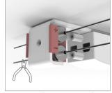
6. Insert the + wire in the + terminal and the - wire in the - terminal.
