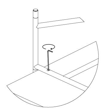
Using the hex key only, turn each screw slightly into the thread so it is secure. Do not screw tightly until all screws are placed in the holes.
