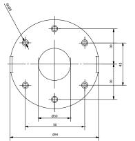
1. Attach wall plate by using 4 screws (included) Make sure that the plate is mounted straight.
